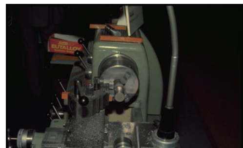
Figure 2: dreborid-B during the turning of a metal-powder coated steel component
