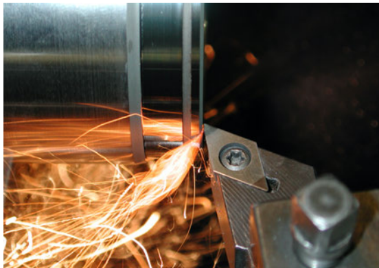
Figure 1: »CBN-DUO-power« in action – Turning instead of grinding
