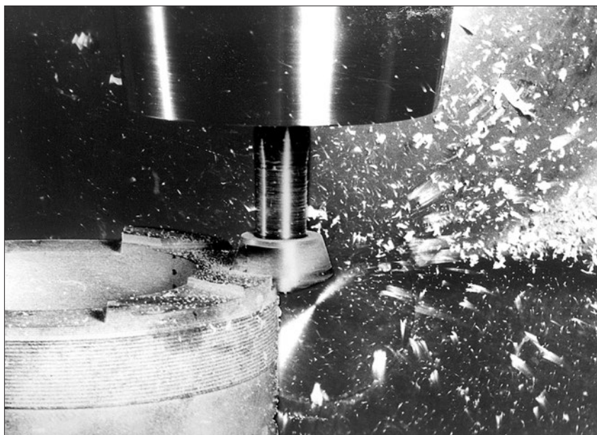
1974 – LACH DIAMANT® demonstrates for the first time the milling of plastics and aluminum with PCD at the Hanover spring trade show (image shows machining of GRP)
