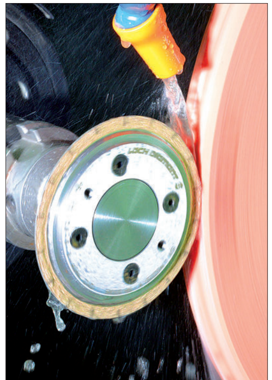
2016 – GrindTec Augsburg: introduction of “drebojet®-plus” as another example of non-stop innovations; contour-controlled dressing of conventional grinding wheels at LACH DIAMANT®’s booth
