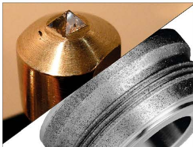
Diamond contra diamond; for example a single natural diamond dresser compared to a diamond dressing roll
