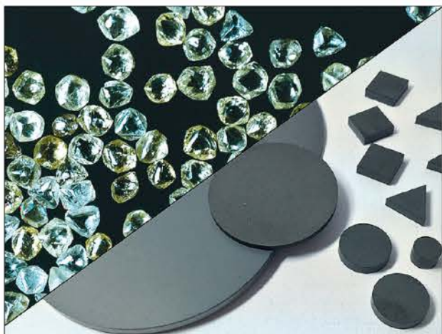
Diamond contra diamond – for example, natural diamond compared to polycrystalline diamond blades (PCD)
