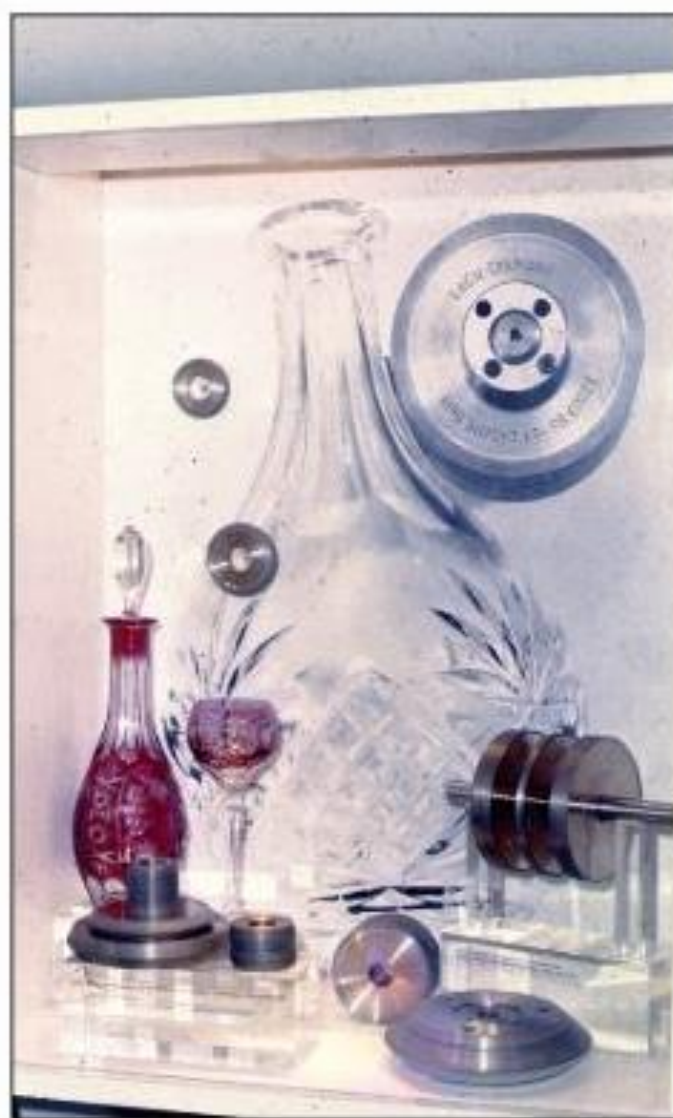
During the boom of the 60's: metal-bond diamond grinding wheels for automated cutting of crystal glasses on Kutscher machines.
