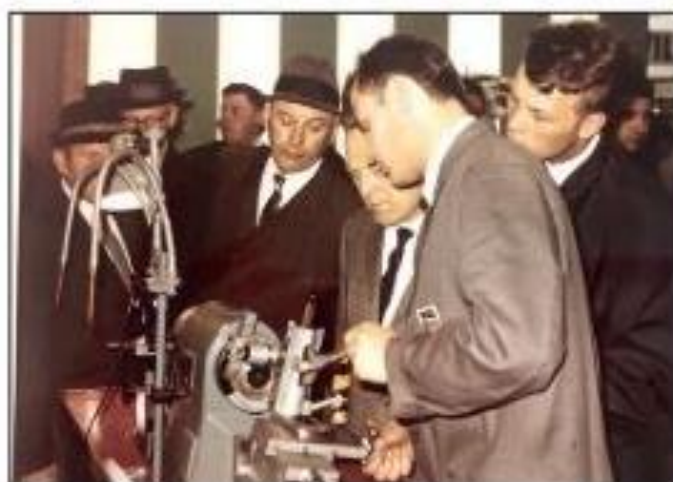
At Hanover trade show in 1968, and to an astonished audience of experts, Karl Ruth demonstrates cutting with a newly-developed resin-bond diamond grinding wheel (K-MC bond) with a metal-coated diamond grain on a Simon steel grinding machine
