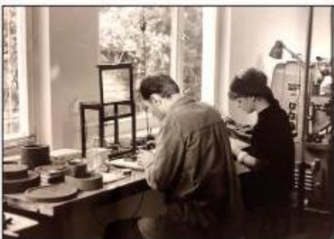
A view into part of the diamond wheel production in the mid-sixties: Ute Kiesel and Karl Ruth in the process of filling wheel forms
