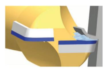
Cool Injection cools the hot chip specifically after it has formed through the opened rake face of the PCD cutting edge.
