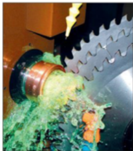
Example: grinding of diamond saw blades with a programme for multi-production
