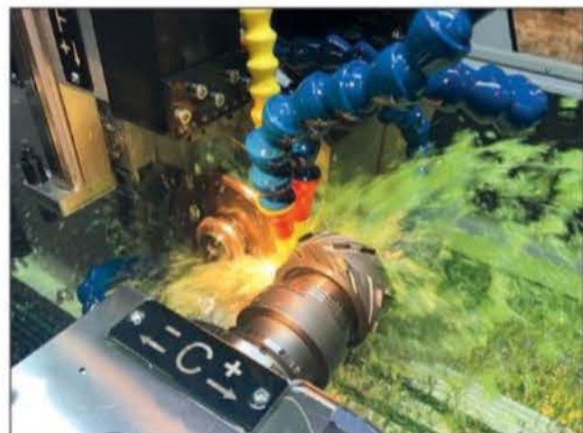
Diamond joint milling cutter with extreme axis angles during sharpening on a «Dia-2200-mini» machine
