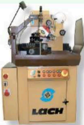
Precision steel grinding machine, model «pcd-100» with rocker for grinding PCD and PCBN inserts and turning steels with diamond grinding wheel
