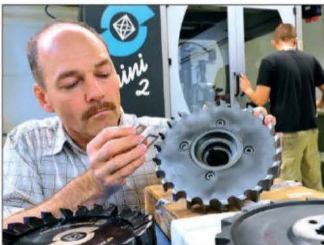
Inspection of a PCD monoblock milling cutter
