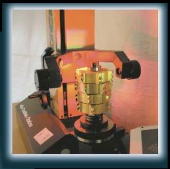
The chief attraction of this tool editor is its ability to communicate directly with the measuring software of the camera measuring system! All the measured cutting positions are automatically recorded in the tool editor. Manual transfer, the writing and typing in of data, which is usual for example with normal measuring devices where it represents a major source of errors, does not exist with the "dia-ToolNet" station.
