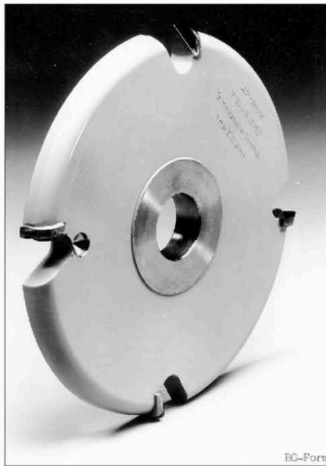
figure 7 and 8 After examination, a diamond profil milling cutter was marked "BG-Form" back then - today "BG-Test"
