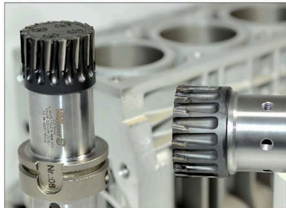
figure 9 A view into the future of machining aluminium in the automobile industry - diamond monoblock cutter Z=16 with cool injection and chip breaker
