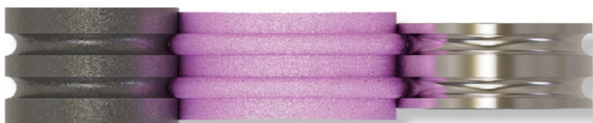
Example of bearing industry: bearing tracks of high-precision bearings (inner rings)
