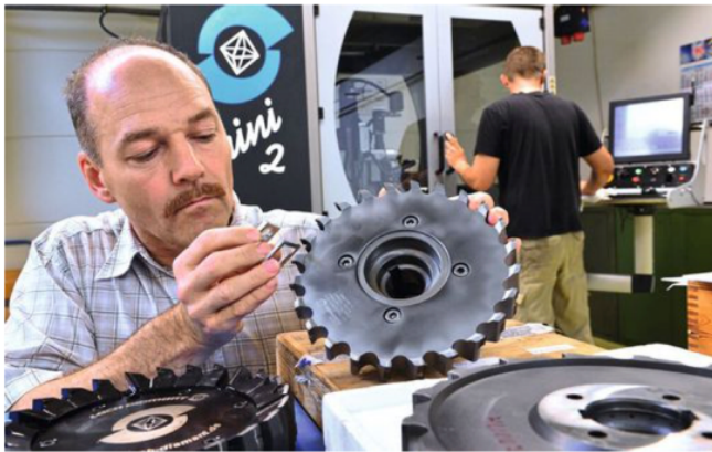
Inspection of a PCD monoblock milling cutter.
