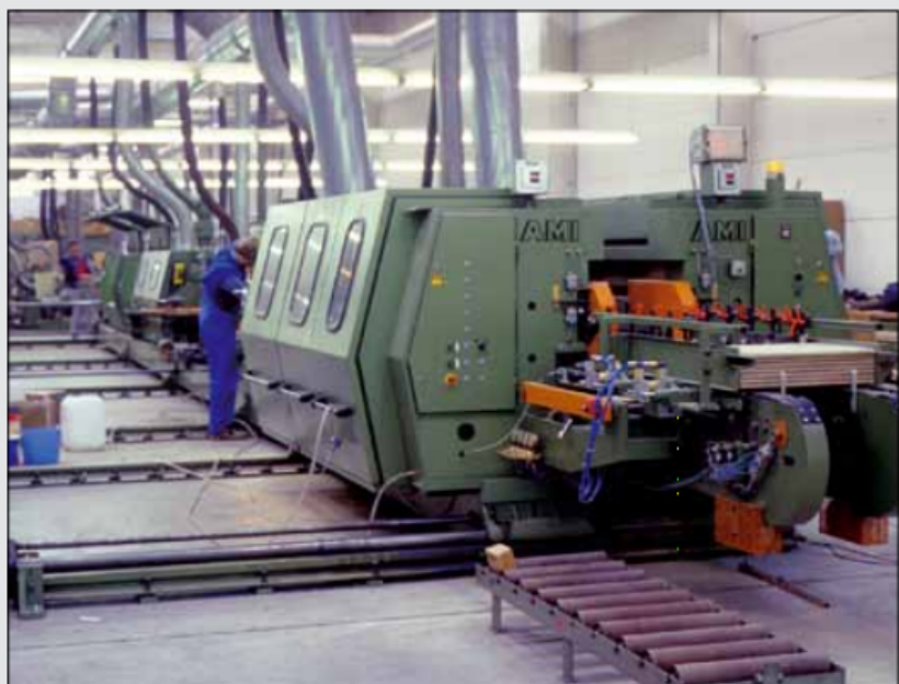
Example of a postforming facility.
