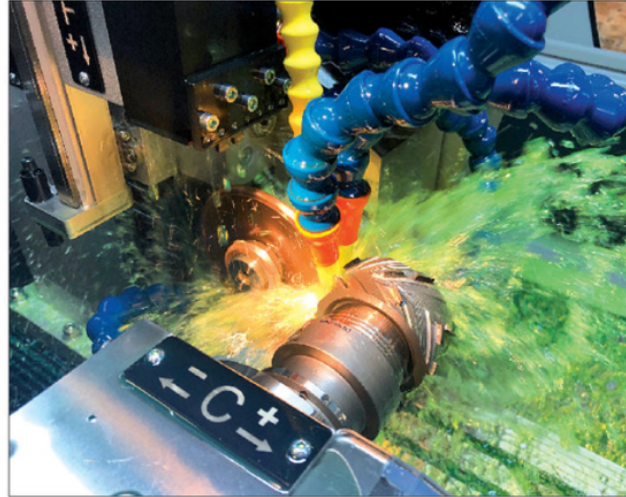
«Dia-2200-mini» during grinding operation - multiple manufacturing possible
