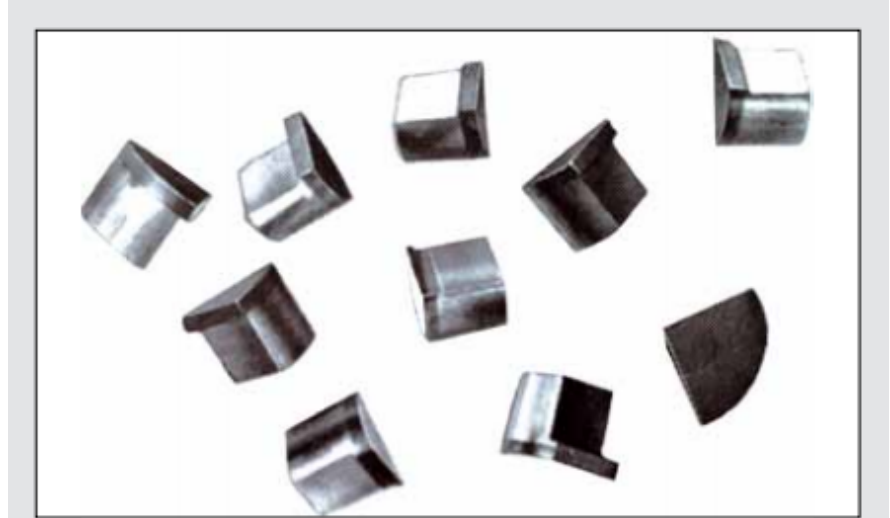
Unmachined synthetic cutting inserts – developmental status as of 1973. The shown segments with 60° and 90° angles were mechanically cut out of PCD blanks (of approx. ø 3.4 mm) with diamond cutting wheels.
