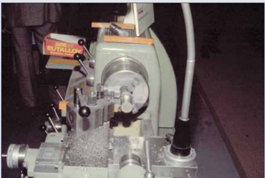
dreborid-G-AS during turning of a metal powder coated steel part.
