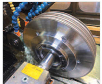
Revolutionary deep grinding with «contour-profiled», metal-bond diamond and CBN profile grinding wheels - showing a CBN grinding wheel (© 400 mm) on a mini «contour-profiled» spark grinding machine EDG-plus
