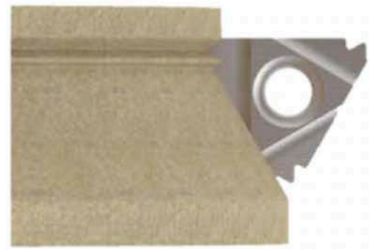
Schematic picture of a metal bond diamond profiling grinding wheel, »contourprofiled«, during deep grinding of a threading insert – Cost efficient: 1 instead of 3!
