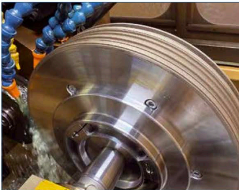
Example of a multi-part »contour-profiled« metal bond CBN grinding wheel, \varnothing 400 x 110 mm, on an »EDG-plus-mini-contour-profiled« EDG sharpening machine – during service, profiles can be resharpened with highest precision and repeatable quality for high tool times.
