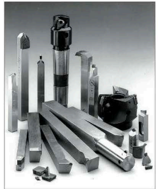
Successful polycrystalline diamond tools of the first hours – examples (1973 - 1974)
