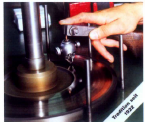
Cutting of industrial diamonds as an example for services for single-point diamond dressers and profile shaped diamond tools
