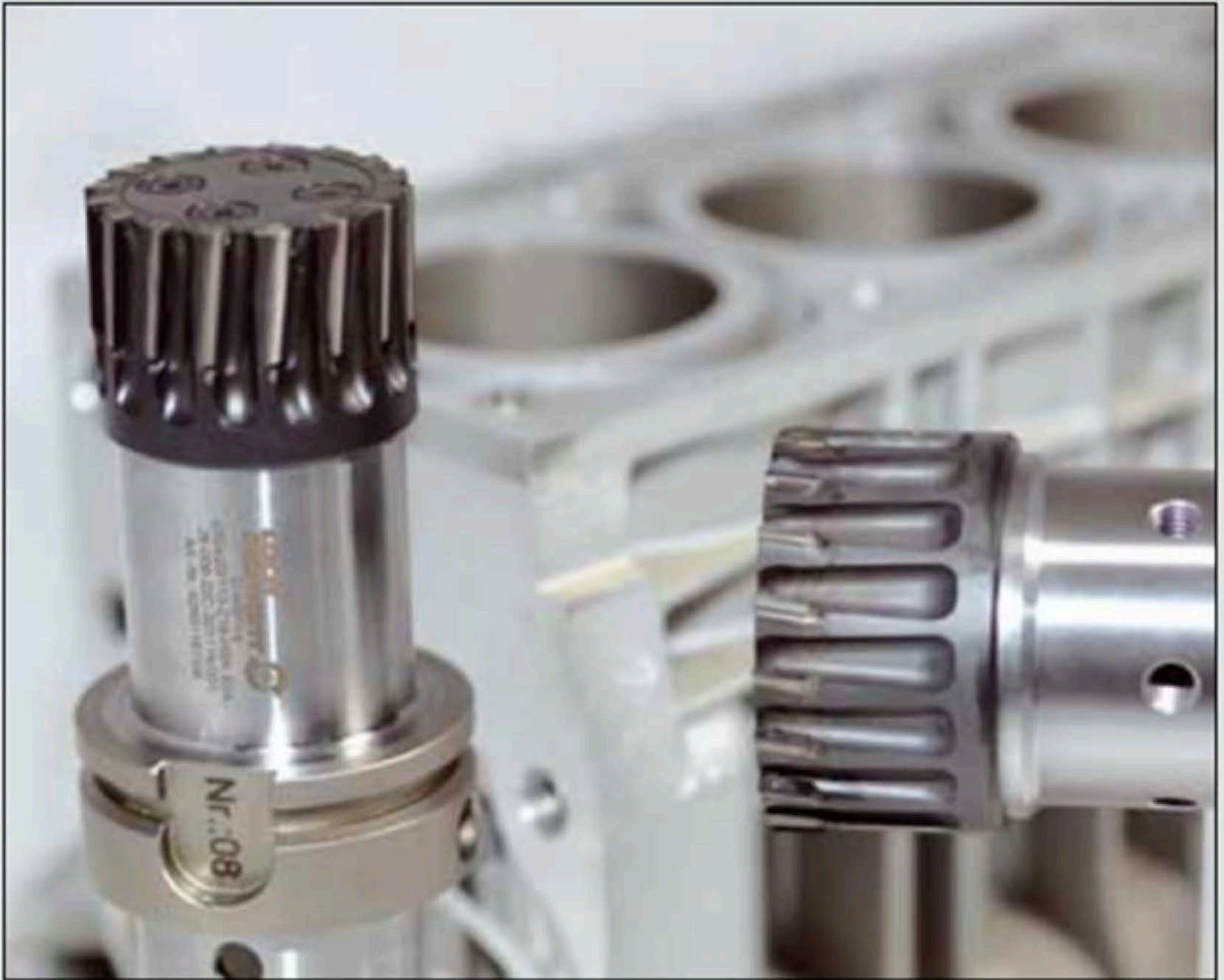
Image 9: A view into the future of machining aluminium in the automobile industry: Diamond Monoblock cutter Z = 16 with cool injection and chip breaker.
