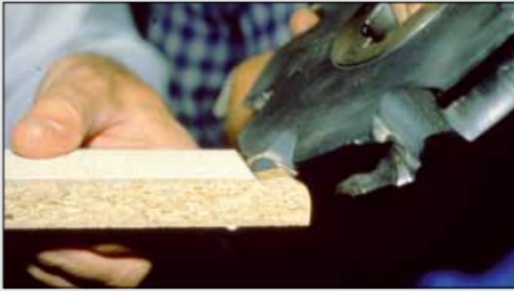
LACH DIAMANT dreboform® profile milling cutter for coated decorative plates.
