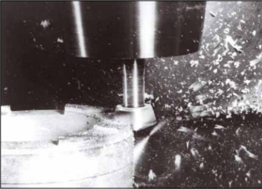
Chip generating PCD milling of glass fibre reinforced plastic (GRP) at experiment in 1974.
