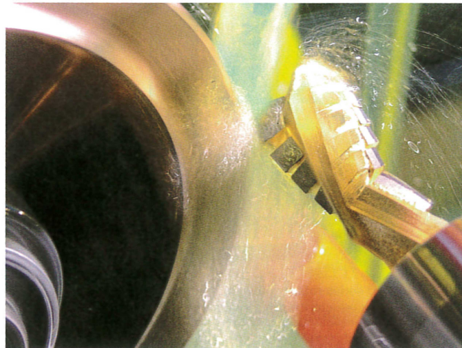
The PCD milling cutter with extreme axial angles for processing wood and composite materials – precisely sharpened on a Dia-2200-mini.
