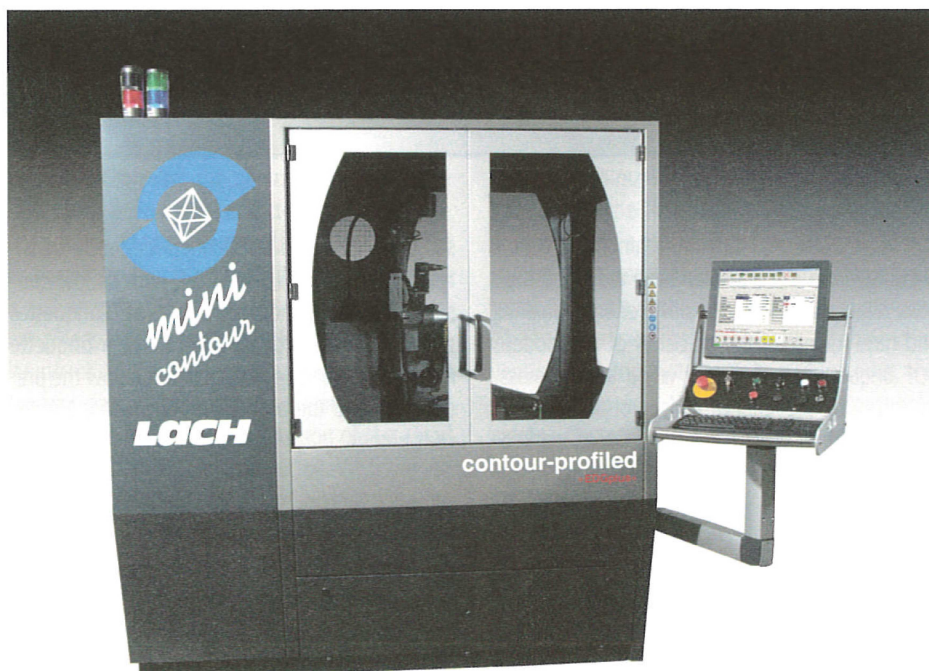
Special model "Dia-contour-profiled" for precise profiling of metal-bond diamond and CBN grinding wheels.
