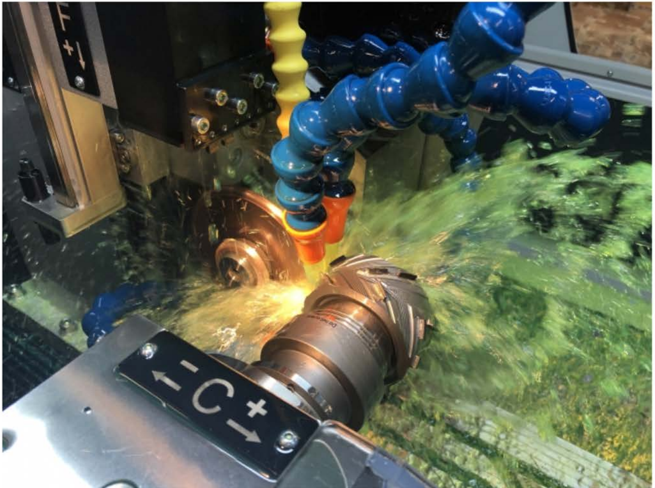
Demonstration of LACH-EDG spark erosion grinding on a »Dia-2200-mini«.
