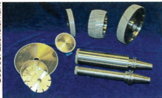
Examples of electro-plated diamond and CBN tools.
