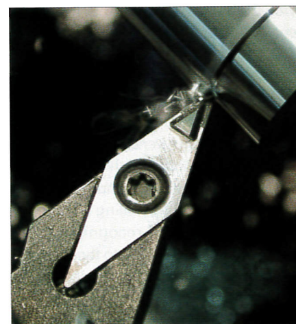
Fig 4 (top) The latest development from Lach: the monoblock cutter for machining aluminium
