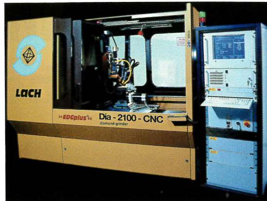
Fig 3 (left to right) CNC machine for machining one and two sides of the flanks of saw blades in one set-up; the PCD diamond universal grinding machine M-1050-automatic, first launched at Ligna '87; the Dia-2100-CNC developed for the grinding of all diamond tools used in the wood and plastics industries
