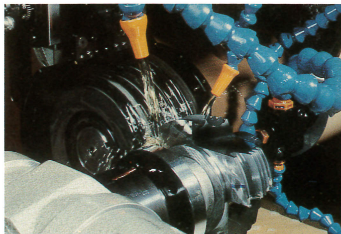
▲ Generating the form on a Drebojet diamond mill dressing roll using a Lach M-1050 automatic machine incorporating the original Lach EDG process.
