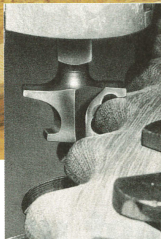
Polycrystalline diamond tools have won a firm place for themselves in modern-day woodworking; the photo shows diamond tools for routing work
