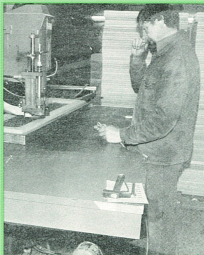
Far left: The Bentrup plant of the CS-Collection Stil Corp. uses diamond tooling on its Japanese-made Heian router. Left: The company manufactures primarily high-end living room period furniture of solid American red oak.
