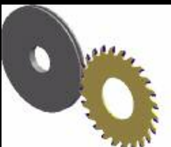
Sharpening of diamond scoring tools for laminates for printed circuit boards (PCB)
