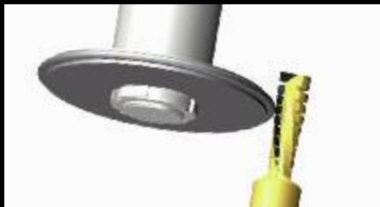
Diamond router bits – shear angle
