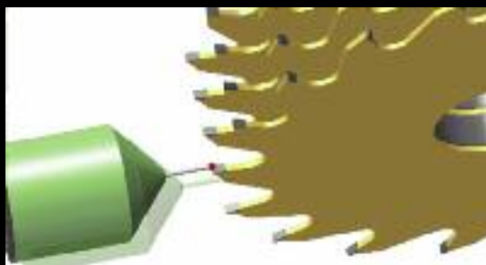
Multiple manufacturing of diamond tools in one clamping, for example circumferential saws
