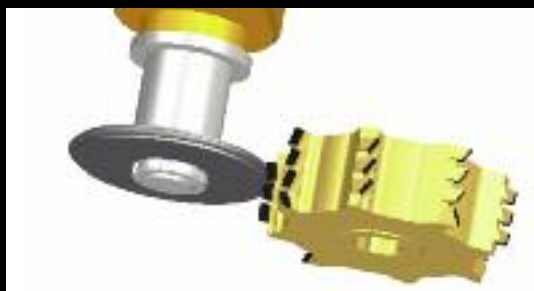
Diamond jointer tools – shear angle
